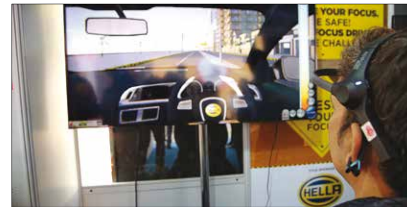
Hella India's Virtual Reality simulator judges a user's alertness level while driving on a scale of 0 to 500. The VR 'game' also prompts the user to adopt good driving habits.
